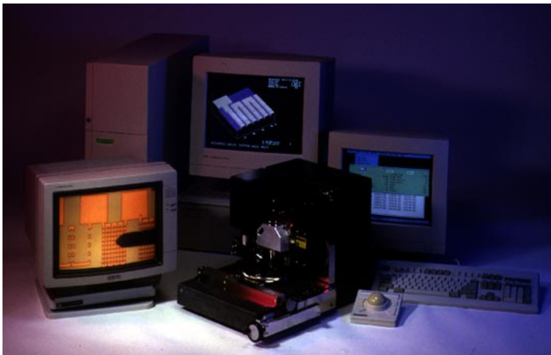
FIGURE 2. LABORATORY SETUP OF THE DIMENSION 3000 SPM INCLUDING THE SCANNER, SAMPLE DISPLAY SCREEN, CONTROL SCREEN, PROCESSOR, AND IMAGE DISPLAY SCREEN (PHOTO COURTESY DIGITAL INSTRUMENTS, SANTA BARBARA, CA).
